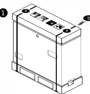
Cut all the straps (a) from the unit using strap cutter(b) as shown in figure.
