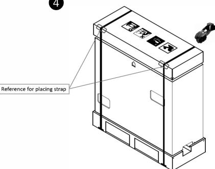
Fix the straps (a) on the unit with help of strap • fixing machine (f) as shown in figure. Use marked reference for placing straps)
