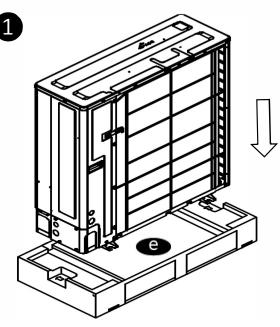
Cover the unit with polythene product cover, then pick the unit up and settle it down on the bottom skid(e) as shown in figure.
