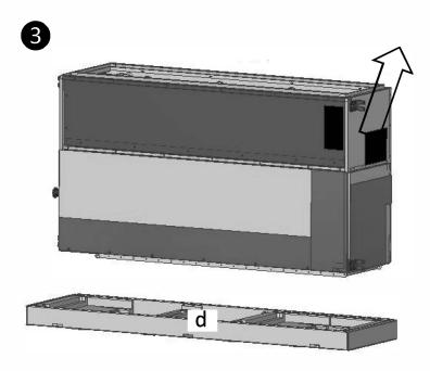
Remove the bottom corrugated cardboard sheet(d) & EPS from the unit by pulling the unit up as shown in figure, then remove the polythene product cover.
