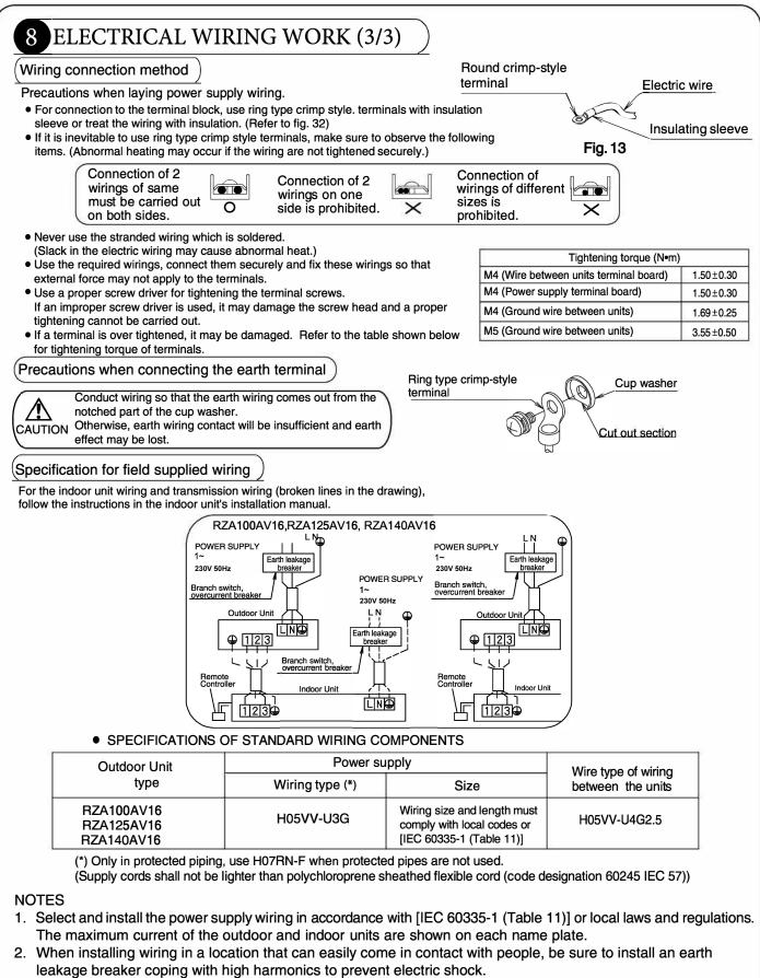
3. Breaker type and capacity shall be selected in accordance with local laws and regulations.
