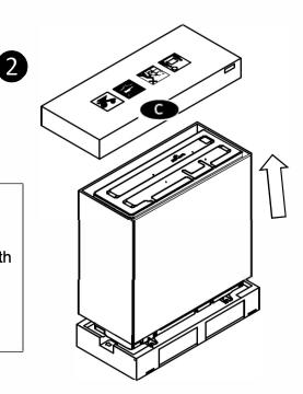
Remove the Top corrugated cardboard sheet with EPS from the unit by pulling it up as shown in figure.
