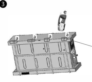
• Fix the straps (a) on the unit as shown in figure.(Use marked reference for placing straps)
