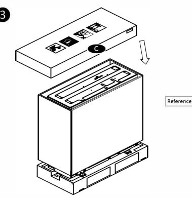
Put the top corrugated cardboard sheet and EPS (c) on the top of the unit as shown in figure.
