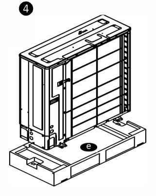
Remove the bottom skid(d) with EPS by pulling the unit up, then remove the polythene product cover by pulling it up
