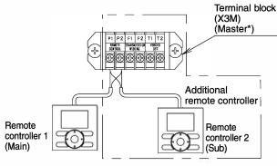
\* For simultaneous operation system, be sure to connect the remote controller to the master unit.
