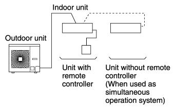
• Heat pump type This system provides COOLING, HEATING, AUTOMATIC, PROGRAM DRY, and FAN OPERATION modes.
