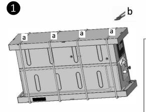
Cut all the straps (a) from the unit using strap cutter(b) as shown in figure.
