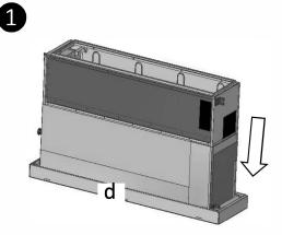
Cover the unit with polythene product cover, then pick the unit up and settle it down on the bottom corrugated cardboard sheet with EPS(d) and cover the unit with polythene product cover as shown in figure
