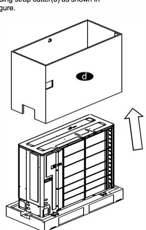
Remove the cardboard box from the unit by pulling it up as shown in figure.
