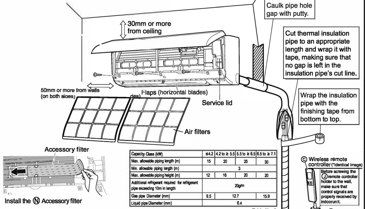
\* Be sure to add the proper amount of additional refrigerant. Failure to do so may result in reduced performance.
