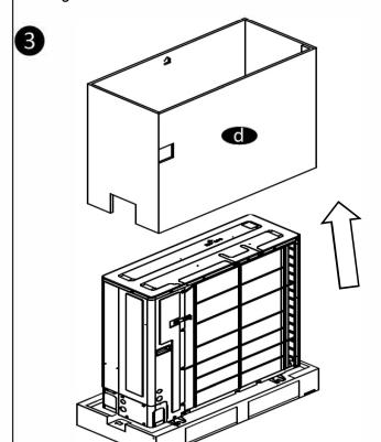
Remove the cardboard box from the unit by pulling it up as shown in figure.
