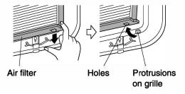
(2) Lift the air filter and remove the holes of the air filter from the protrusions on the upper side of the grille. (Both left and right sides.)
