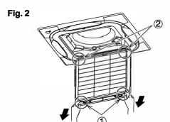
Pull the ends of the air filter down and remove the holes of the air filter from the grille protrusions. (Both left and right sides.)
