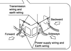
When wiring, using single core wires for the earth wiring, tie the power supply wiring and the earth wiring by clamp material as shown in the right figure.
