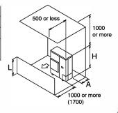
3-2 IN CASE OF INSTALLING MULTIPLE UNITS (2 UNITS OR MORE) IN LATERAL CONNECTION PER ROW (Units: mm)
