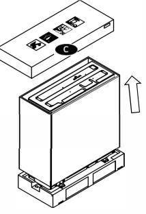
Remove the Top corrugated cardboard sheet with EPS from the unit by pulling it up as shown in figure.
