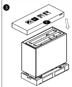
Put the top corrugated cardboard sheet and EPS (c) on the top of the unit as shown in figure.
