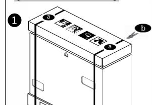
Cut all the straps (a) from the unit using strap cutter(b) as shown in figure.
