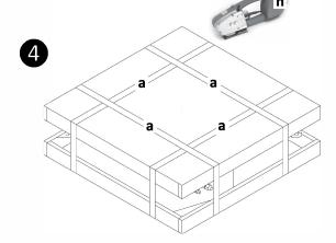
Cut all the straps (a) from the unit using strap cutter (b) as shown in figure.
