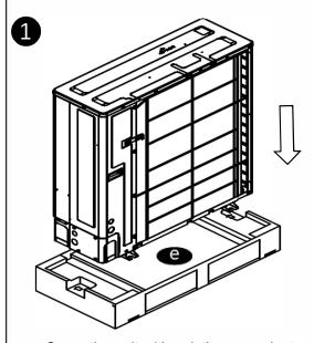
Cover the unit with polythene product cover, then pick the unit up and settle it down on the bottom skid(e) as shown in figure.
