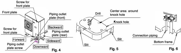
• After knocking out the knock hole, it is recommended to apply repair paint to the edge and the surrounding end surfaces to prevent rusting.
