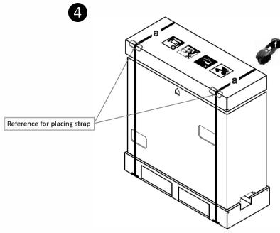
Fix the straps (a) on the unit with help of strap fixing machine (f) as shown in figure. (Use marked reference for placing straps)
