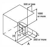
Pattern 2) Where obstacles in front of the outlet side is lower than the outdoor unit
