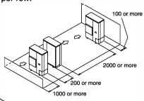
(2) In case of installing multiple units (2 units or more) in lateral connection per row.
