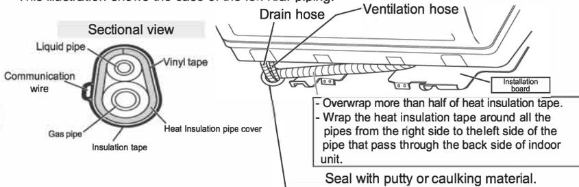
Fill the gap from both the indoor side and the outdoor side to prevent dew condensation, misdetection of indoor temperature, and invasion of small animals.
