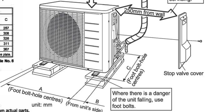
In sites with poor drainage, use block bases for outdoor unit. Adjust foot height until the unit is leveled. Otherwise, water leakage or pooling of water may occur.
