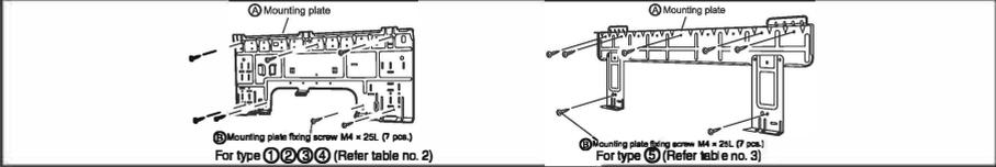
Note: Before installation, mounting plate size & shape must be matched with mounting plate available in the unit, then accordingly follow the installation instruction.
