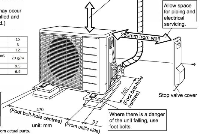
In sites with poor drainage, use block bases for outdoor unit. Adjust foot height until the unit is leveled. Otherwise, water leakage or pooling of water may occur.
