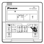
Press the air flow direction button to select the air direction.
