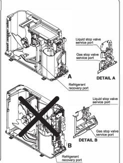
Be sure to write down the additional amount of refrigerant charged or the entire amount re-charged on the precaution plate on the rear of the front panel, as this information is needed in case of after-sales service.
