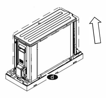
Remove the bottom skid(d) with EPS by pulling the unit up, then remove the polythene product cover by pulling it up
