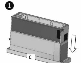
Cover the unit with polythene product cover, then pick the unit up and settle it down on the bottom corrugated cardboard sheet with EPS(d) and cover the unit with polythene product cover as shown in figure
