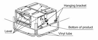
Feed water into the tube and set the indoor unit to the water levels on the left and right.
