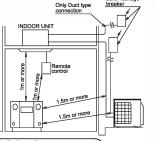
Inverter air conditioners may cause noise to occur in electrical appliances. As shown in the right drawing, select an installation site well away from radios, PCs, and stereos. Especially in the areas where the incoming signal strength is weak, keep the indoor remote controller 3 meter or more from electrical appliances. Put the power supply and transmission wining in a metal piping and ground the metal piping.
