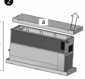
Remove top corrugated cardboard sheet(c) & EPS from the unit by pulling it up as shown in figure.
