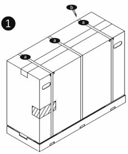
Cut all the straps (a) from the unit using strap cutter(b) as shown in figure.
