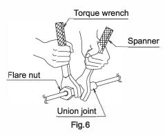
Coat the flared inner surface only with ether oil or ester oil
