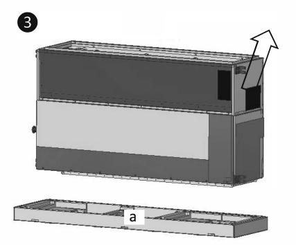
□ Remove the bottom corrugated cardboard sheet(d) & EPS from the unit by pulling the unit up as shown in figure, then remove the polythene product cover.
