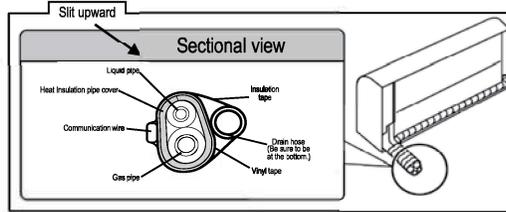
Wrap vinyl tape with the slit of the heat insulation pipe cover facing up so that there are no gap . If there is a gap or if it is tightened too much, it may cause condensation or water dripping.
