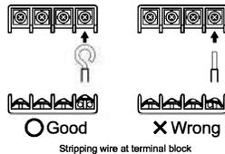
• Precaution to be taken for power supply wiring.
