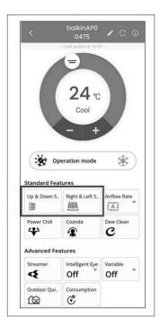
Up & Down Swing and Right & Left Swing will turn to blue in colour which indicates that swing is turn On.User can Turn ON 3D Swing by clicking Up & Down Swing and Right & Left Swing.
