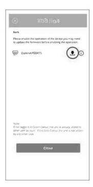
Tap on firmware update button right next to the unit name to update the firmware of AC Wi-Fi.
