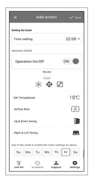
User can now select Time (24Hr format), Unit ON/OFF, Mode(Cool, Fan, Dry) Set Temperature, Fan Speed, Swing. After selecting required setting, user need to Save the setting (Top Right Side).
