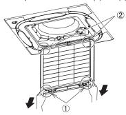
Pull the ends of the air filter down and remove the holes of the air filter from the grille protrusions.
