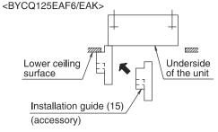
• Apply the long side of the cut-out section in case of designer grille.
