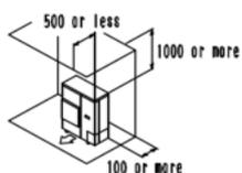
(2) In case obstacles exist in front of the inlet side and on both sides of the outdoor unit,
