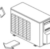
Set the outlet side at right angle to the direction of the wind.
