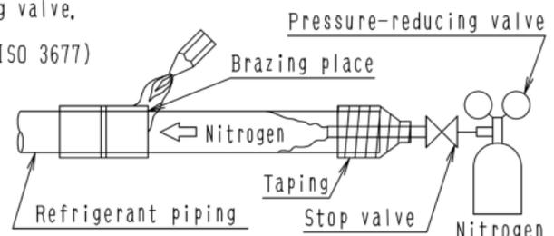
**Prohibited** Do not use anti-oxidants when brazing the piping joints. (Residue can clog pipes and break equipment.)
