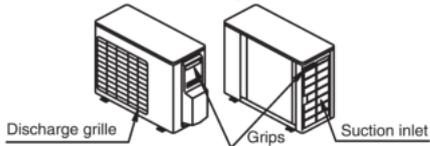
Place your hands on the corner instead of holding the suction inlet in the side of the casing, otherwise the casing could be deformed.
