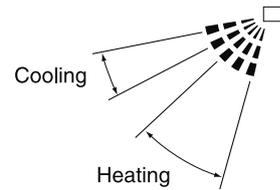
We recommend using the fan in the position shown above when fixing the fan direction.
