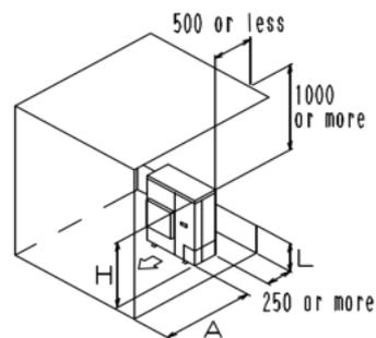
**Pattern 2** Where obstacles in front of the outlet side is lower than the outdoor unit.
