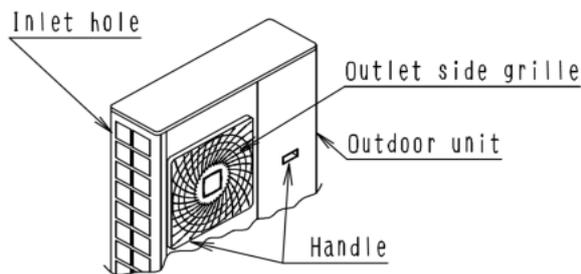
When lifting up the unit, do not put fingers into the inlet hole on the side of the casing, otherwise the casing may be deformed.
