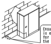
Set the outlet side at a right angle to the direction of the wind.
