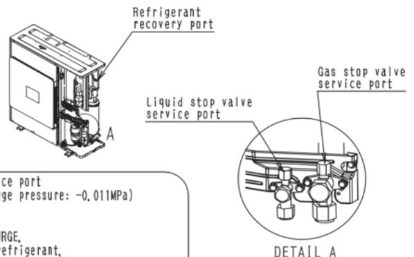
Be sure to write down the additional amount of refrigerant charged or the entire amount re-charged on the precaution plate on the rear of the front panel, as this information is needed in case of after-sales service.
