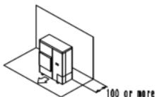
(2) In case obstacles exist in front of the inlet side and on both sides of the outdoor unit,
