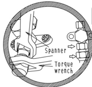
**Do not apply force to the valve cap or the valve body**
