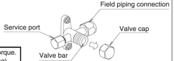
When tightening the flare of the stop valves, make sure to tighten by the rated torque. The rated torque is shown on **CAUTION FOR FLARE CONNECTION** (Following)
