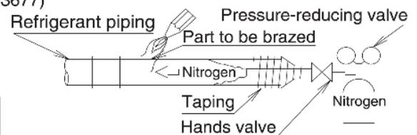
**Prohibited** Do not use anti-oxidants when brazing the piping joints. (Residue can clog pipes and break equipment.)
