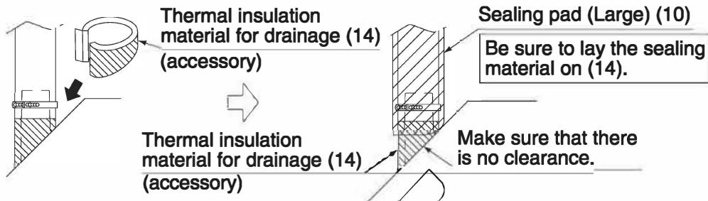
**WHEN ELECTRIC WIRING WORK IS NOT FINISHED**
