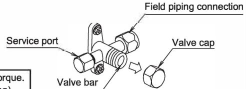
When tightening the flare of the stop valves, make sure to tighten by the rated torque. The rated torque is shown on **(CAUTION FOR FLARE CONNECTION)** (Following)
