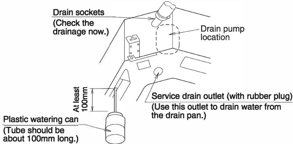
**<Adding water through air discharge outlet>**
