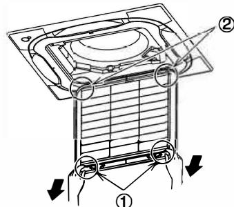
(1) Pull the ends of the air filter down and remove the holes of the air filter from the grille protrusions. (Both left and right sides.)
