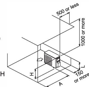
Pattern 2 When the obstacle on the discharge side is lower than the unit
