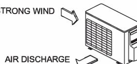
Set the outlet side at right angle to the direction of the wind.
