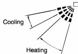
We recommend using the fan in the position shown above when fixing the fan direction.
