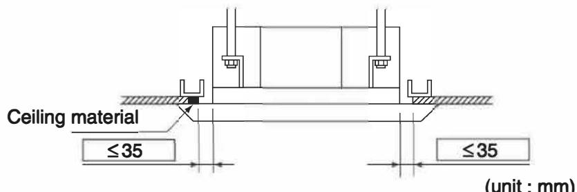
**(2) Make the ceiling opening needed for installation where applicable. (For existing ceilings)**
