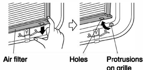
(2) Lift the air filter and remove the holes of the air filter from the protrusions on the upper side of the grille. (Both left and right sides.)
