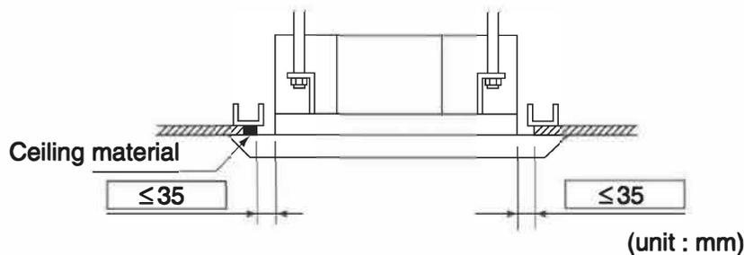
**(2) Make the ceiling opening needed for installation where applicable. (For existing ceilings)**
