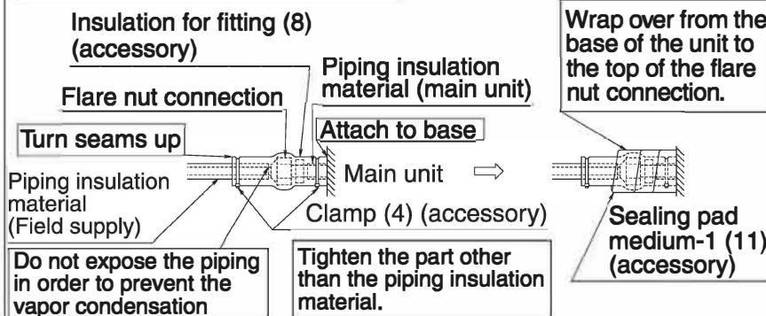
**Liquid Piping Insulation Procedure**
