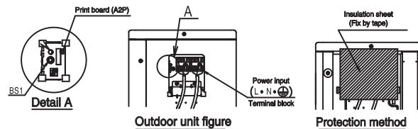
To prevent electric shock when inspection, protect by use insulation sheet on power input terminal block and print board (A2P)
