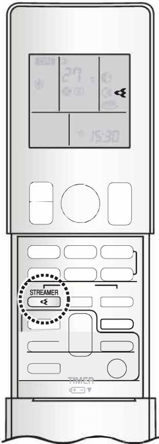
The absorption power of the accessory filter and the decomposition power of the streamer discharge combine to reduce unpleasant odours and viruses, cleaning the air in the room.
