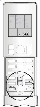
Timer functions are useful for automatically switching the air conditioner on or off in the morning or at night. You can also use the ON TIMER and OFF TIMER together.
