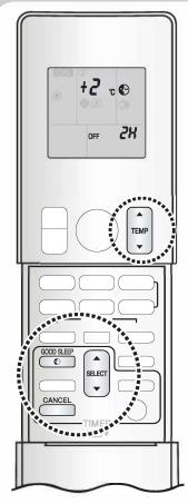
You can prevent excessive cooling of the room during sleep by setting a temperature shift value. The air conditioner automatically stops after the preset time has elapsed, thereby conserving electricity.
