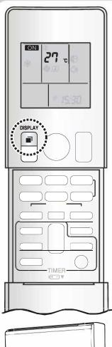
The inverter output and temperature display for the indoor unit shows the current inverter output, indoor temperature, and set temperature.
