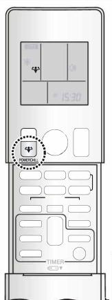
POWER CHILL operation quickly maximises the cooling effect in any operation mode. In this mode, the air conditioner operates at maximum capacity.
