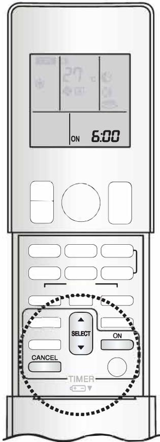
Timer functions are useful for automatically switching the air conditioner on or off in the morning or at night. You can also use the ON TIMER and OFF TIMER together.
