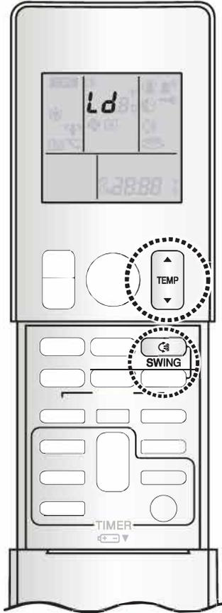
The brightness of the indicator lamp / 7 Segment can be adjusted H(high), L(low), or OFF.
