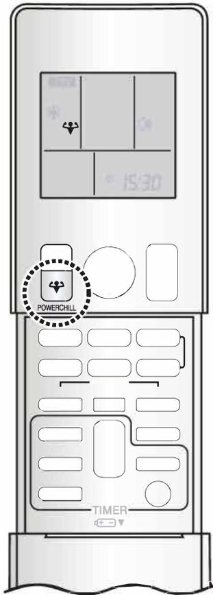
POWER CHILL operation quickly maximises the cooling effect in any operation mode. In this mode, the air conditioner operates at maximum capacity.
