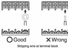
• Precaution to be taken for power supply wiring.
