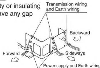
When wiring, using single core wires for the earth wiring, tie the power supply wiring and the earth wiring by clamp material as shown in the right figure.
