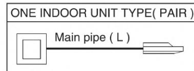
When piping length exceeds its of a top table, or only when you perform recharging, Please be correctly charged according to the following. For future servicing, please describe the amount of additional refrigerant charging, or the amount of recharging in the collective label in accessory set or back side of right side plate.
