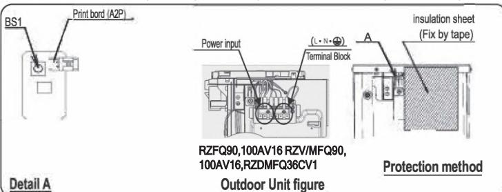
**Caution** To prevent electric shock when inspection, protect by use insulation sheet on power input terminal block and print board(A2P)
