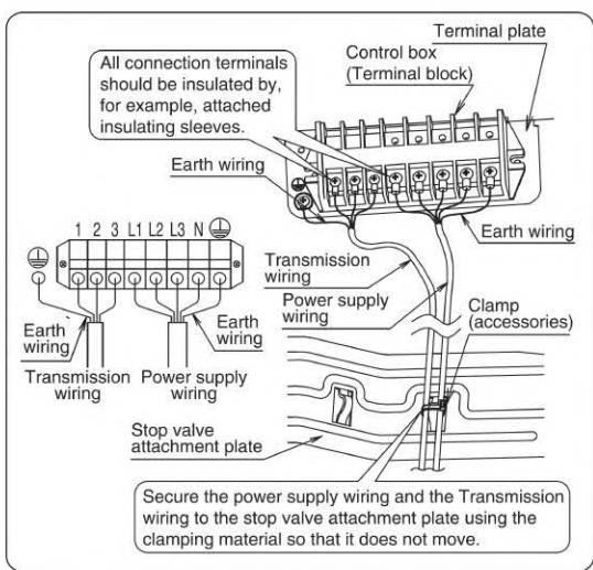
Direction for pulling out the wiring
