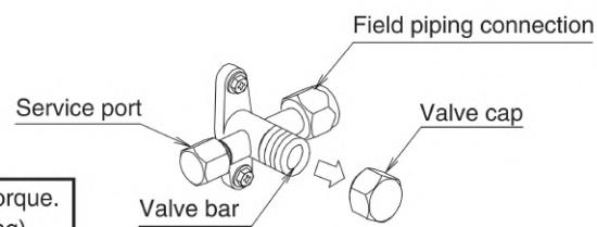
**DO NOT APPLY FORCE ON THE VALVE CAP, THIS MAY RESULT IN A REFRIGERANT LEAK.**
