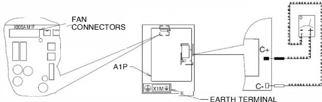
4. After confirming the main circuit capacitor voltage drop, pull out the outdoor unit fan connector, make sure not to touch any live parts during this action. (strong adverse winds which let the outdoor unit fan rotate, induce a risk of electrical shock because the fan rotation makes the capacitor store electricity.
