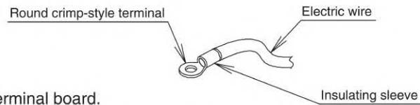
When connecting wires of the same gauge, connect them according to the below figure.
