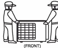
Place your hands on the corner instead of holding the suction inlet in the side of the casing, otherwise the casing could be deformed.
