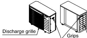
Place your hands on the corner instead of holding the suction inlet in the side of the casing, otherwise the casing could be deformed.
