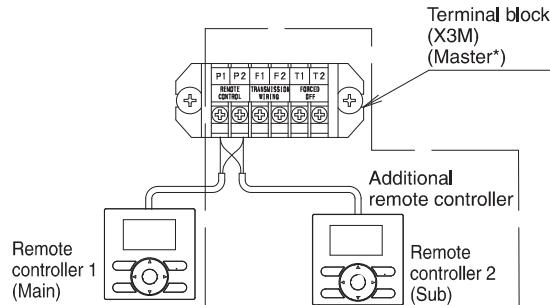
\* For simultaneous operation system, be sure to connect the remote controller to the master unit.
