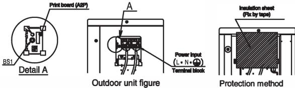
To prevent electric shock when inspection, protect by use insulation sheet on power input terminal block and print board (A2P)
