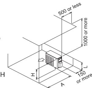
**Pattern 2** When the obstacle on the discharge side is lower than the unit
