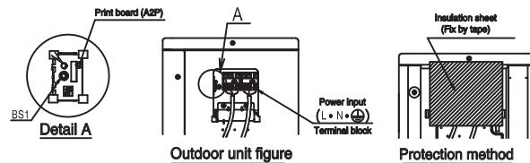
**Caution** To prevent electric shock when inspection, protect by use insulation sheet on power input terminal block and print board (A2P)
