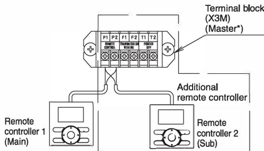
\* For simultaneous operation system, be sure to connect the remote controller to the master unit.
