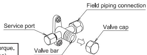
DO NOT APPLY FORCE ON THE VALVE CAP, THIS MAY RESULT IN A REFRIGERANT LEAK.
