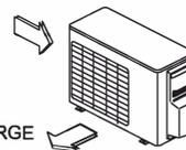
Set the outlet side at right angle to the direction of the wind.
