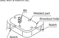
Cutting out the 2 notches makes it possible to carry out installation as shown in the figure below.
