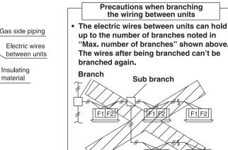
Use 0.75~1.25 mm<sup>2</sup> shielded 2-core wire for the above wiring.
