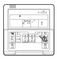
• Press the air flow direction button to select the air direction.
