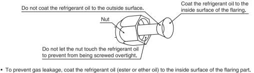
Refer to the following table for the tightening torque. (Being screwed overtight will damage the flaring part.) 32.7~39.9N•m 12.8~13.2mm
