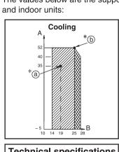
Equivalent piping length...7.5m Difference in height.....0m Outdoor temperature (°CDB) B Indoor temperature (°CWB) Range for continuous operation Range for pull down operation
