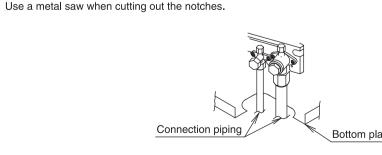
· After drilling through the knockout hole, it is recommended to coat the edges of the notches and the area around them with anti-corrosion paint to prevent rusting.
