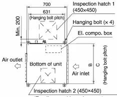
(For disassembly such as motors and drain pan) When work is possible in space of the unit lower part, inspection hatch 2 is unnecessary.
