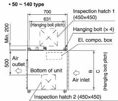
(For disassembly such as motors and drain pan)
