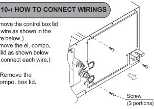
(2) Lay the wires in the el. compo. box through the wire inlet on the side of the el. compo. box.
