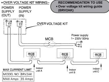
FUNCTION:-IT IS USED TO PROTECT FROM OVER VOLTAGE AND UNDER VOLTAGE CONDITION.
