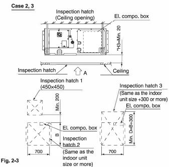
Axial direction view A-1 Axial direction view A-2  Determine the H3 dimension by maintaining a downward slope of at least 1/100 as specified in "7. DRAIN PIPING WORK".
