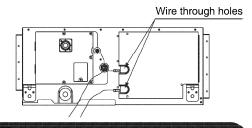
After all the wiring connections are done, fill in any gaps in the through holes with putty or insulation (procured locally) to prevent small animals and insects from entering the unit from outside. (If any do get in, they could cause short circuits in the el. compo. box.)
