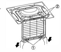
Pull the ends of the air filter down and remove the holes of the air filter from the grille protrusions. (Both left and right sides.)
