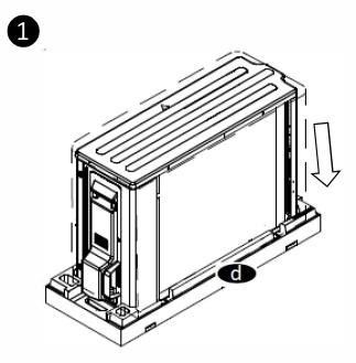
Cover the unit with polythene product cover, then pick the unit up and settle it down on the bottom skid(d) as shown in figure.
