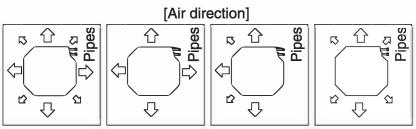
All-round air Four air direction Three air direction Two air direction
