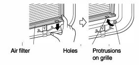
(2) Lift the air filter and remove the holes of the air filter from the protrusions on the upper side of the grille. (Both left and right sides.)
