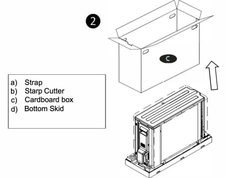
Remove the cardboard box(c) from the unit after opening it and pulling it up as shown in figure.
