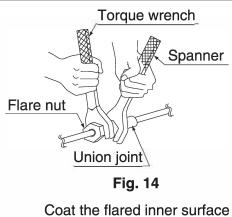
Coat the flared inner surface only with ether oil or ester oil
