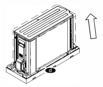
Remove the bottom skid(d) with EPS by pulling the unit up, then remove the polythene product cover by pulling it up
