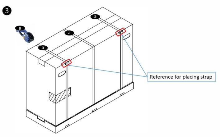
• Fix the straps (a) on the unit by using portable strap fixing machine as shown in figure.(Use marked reference for placing straps)
