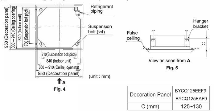
■ Use the installation guide (15) (delivered with the unit) for exact vertical positioning of the unit.
