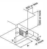
Pattern 2) When the obstacle on the discharge side is lower than the unit
