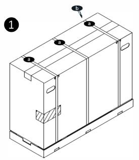
Cut all the straps (a) from the unit using strap cutter(b) as shown in figure.
