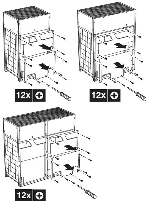
Once the front plates open, the electrical component box can be accessed by removing the electrical component box cover as follows.
