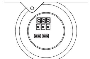
Operate the switches and push buttons with an insulated stick (such as a closed ball-point pen) to avoid touching of live parts.
