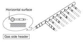
Mount the REFNET header so that the branch pipes are on the underside and branch horizontally.
