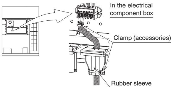
How to pass wire through the rubber sleeve:
