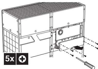
For service purposes, the push buttons on the main PCB need to be accessed. To access these push buttons, the electrical component box cover does not need to be opened. See “13. Making field settings”.
