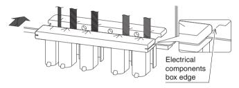
Fix with a clamp.Fix by passing the clamp through the hook on the back.
