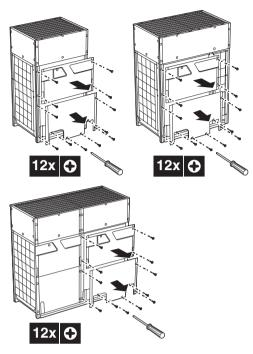
Once the front plates open, the electrical component box can be accessed by removing the electrical component box cover as follows.
