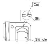
When side connections, remove the through hole cover for punching a hole and return the through hole cover to original place and tighten a screw.
