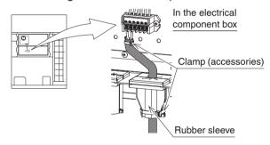
How to pass wire through the rubber sleeve:
