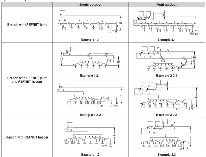
Difference in height between outdoor and indoor units: H1. Difference in height between indoor and indoor units: H2. Difference in height between outdoor and outdoor units: H3.
