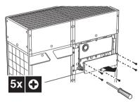
For service purposes, the push buttons on the main PCB need to be accessed. To access these push buttons, the electrical component box cover does not need to be opened. See "13. Making field settings".
