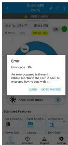
When machine is in error condition like faulty heat exchanger temperature sensor (Error code : C4) etc., a pop-up will show in App that an error occurred in the unit.
