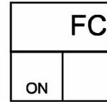
After completion of Filter Clean Indicator duration, IDU display will show "FC" and the Operation LED (Green) and Timer LED (Orange) will blink alternately for 5 minutes, This will indicate to the user that it's time to clean the filters. After cleaning the filters, user needs to reset the filter clean indicator operation by following the process below.
