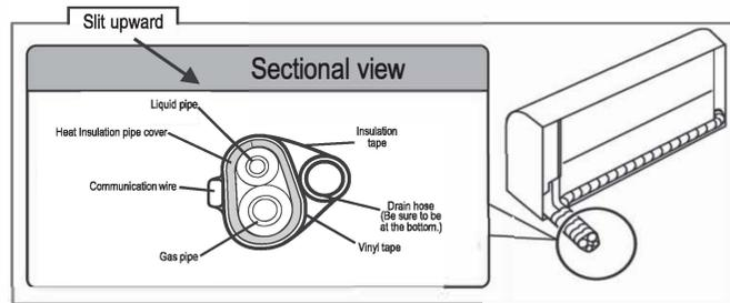
Wrap vinyl tape with the slit of the heat insulation pipe cover facing up so that there are no gap . If there is a gap or if it is tightened too much, it may cause condensation or water dripping.
