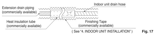
• Make sure the diameter of the piping is the same as the piping (hard vinyl chloride, nominal diameter 13mm) or bigger.
