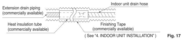
Make sure the diameter of the piping is the same as the piping (hard vinyl chloride, nominal diameter 13mm) or bigger. · When directly connecting a hard vinyl chloride pipe joint (nominal diameter 13mm) to the drain hose connected to the indoor unit (i.e. for embedded piping, etc.), use a commercially available hard vinvl chloride pipe joint (nominal diameter 13mm). (Refer to Fig. 18)
