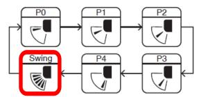
• The left/right airflow direction position switches each time the left/right airflow direction button is pressed.
