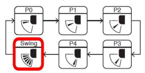
• The left/right airflow direction position switches each time the left/right airflow direction button is pressed.
