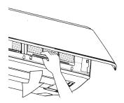
3. Clean the air filter. Use vacuum cleaner A) or wash the air filter
