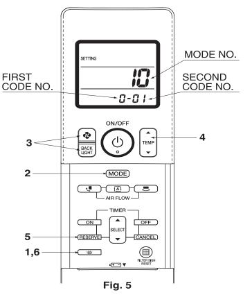
If the time to clean air filter is set to "Filter Contamination-a lot", set MODE NO. to "10", FIRST CODE NO. to "0", and SECOND CODE NO. to "02".
