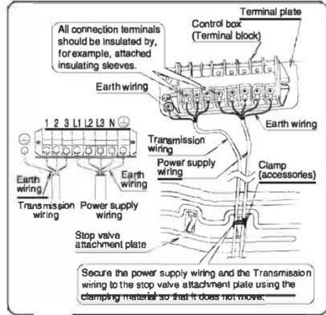
**Direction for pulling out the wiring**
