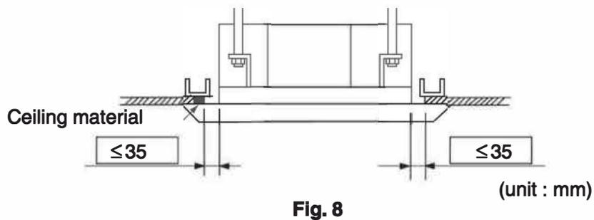
**(2) Make the ceiling opening needed for installation where applicable. (For existing ceilings)**
