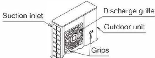
Place your hands on the corner instead of holding the suction inlet in the side of the casing, otherwise the casing could be deformed.
