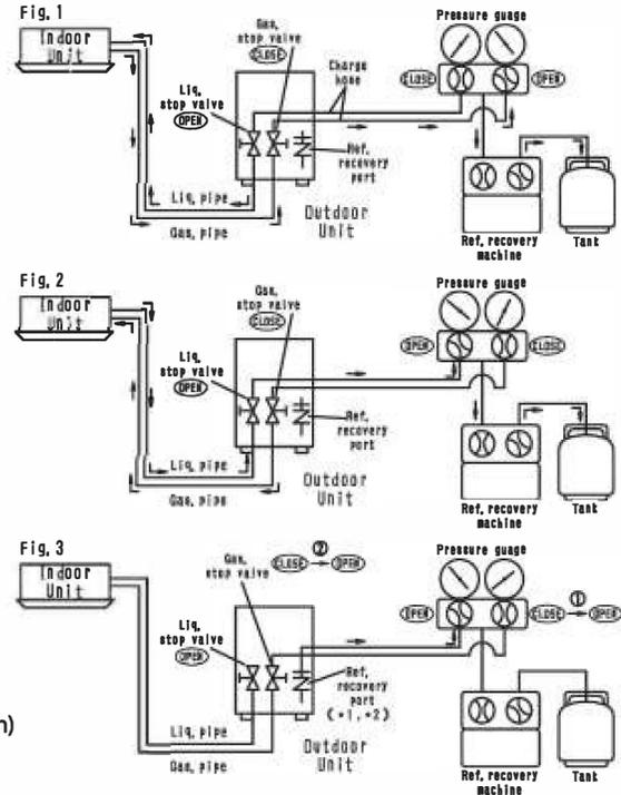
**Retaining oil recovery amount improved approx. 5 times from regular refrigerant recovery method**
