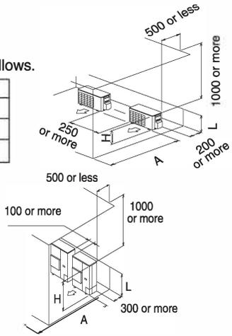
**Pattern 2** When the obstacle on the discharge side is lower than the unit
