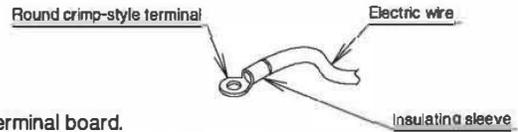
When connecting wires of the same gauge, connect them according to the below figure.
