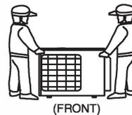
Place your hands on the corner instead of holding the suction inlet in the side of the casing, otherwise the casing could be deformed.
