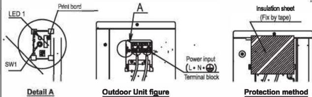
**Caution** To prevent electric shock when inspection, protect by use insulation sheet on power input terminal block and print board (A2P)
