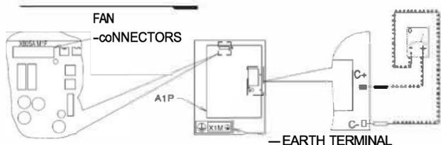
4. After confirming the main circuit capacitor voltage drop, pull out the outdoor unit fan connector, make sure not to touch any live parts during this action. (strong adverse winds which let the outdoor unit fan rotate, induce a risk of electrical shock because the fan rotation makes the capacitor store electricity.)
