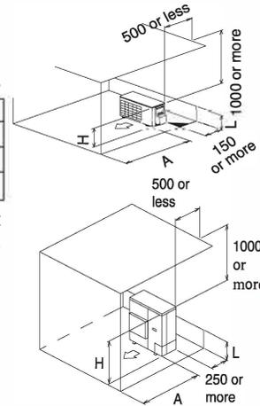
**Pattern 2** When the obstacle on the discharge side is lower than the unit
