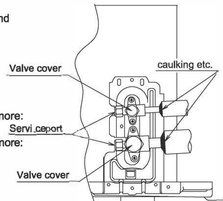
**Caution** Insulation of interunit piping must be carried out up to the connection inside the casing. If the piping is exposed to the atmosphere, it may cause sweating or burn due to touching the piping, electric shocks or a fire due to the wiring touching the piping.
