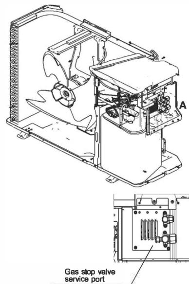
Be sure to write down the additional amount of refrigerant charged or the entire amount re-charged on the precaution plate on the rear of the front panel, as this information is needed in case of after-sales service.
