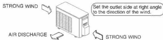
Set the outlet side at right angle to the direction of the wind.
