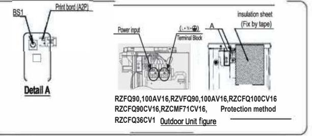
To prevent electric shock when inspection, protect by use insulation sheet on power input terminal block and print board(A2P)
