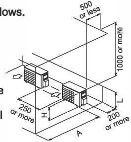
**Pattern 2** When the obstacle on the discharge side is lower than the unit
