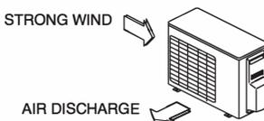
Set the outlet side at right angle to the direction of the wind.
