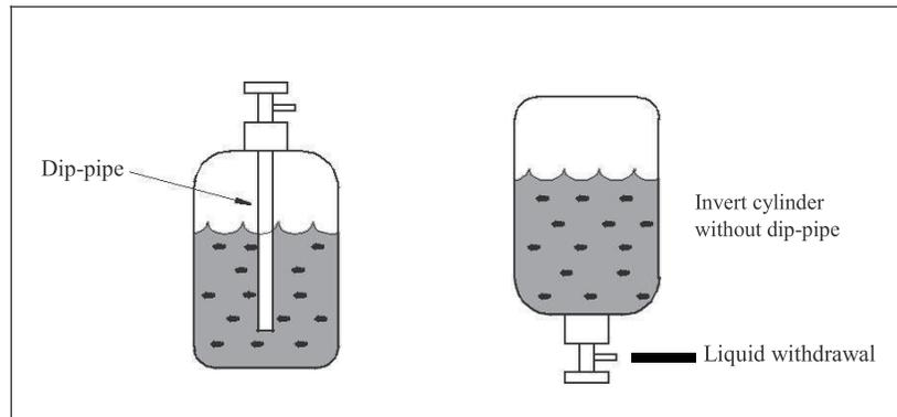
**It recommends charging liquid in a CONTROLLED manner into the suction side until the system is full.**
